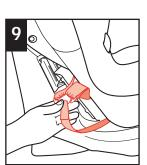
Pull out the harness and splitter plate.
